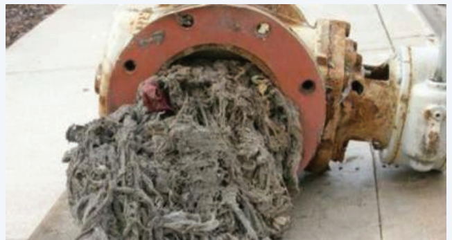
A mass of flushable and disinfectant wipes clogs a pipe.
